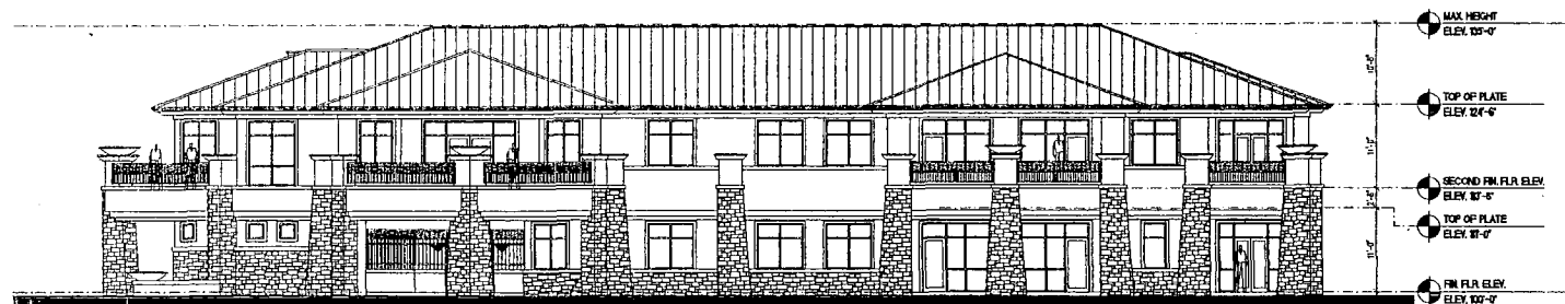
2 WEST BUILDING ELEVATION (FACING RESIDENTIAL) SCALE: 1/8"=1'-0"
