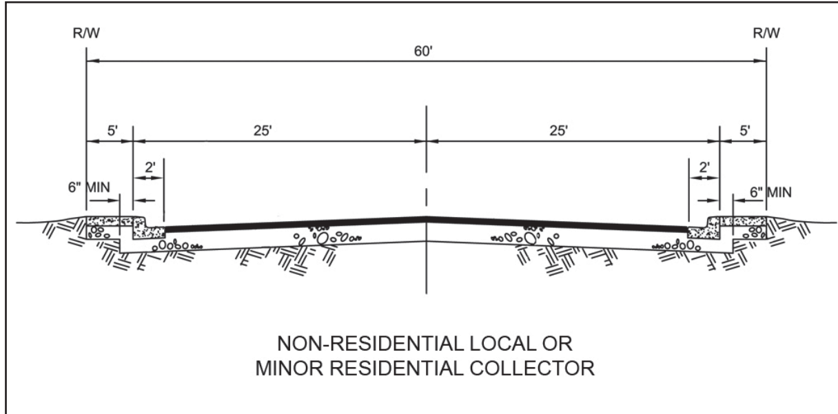
Figure IE: Secondary Thoroughfares, without Detached Sidewalk (60' Width)
