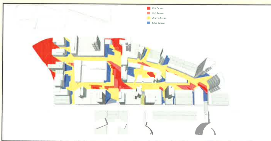
Solar Exposure Analysis- This diagram highlights the hottest areas at 3 pm on Jun 21, as indicated by the red shaded areas. These are the areas that need the most protection from the sun that buildings cannot provide.
