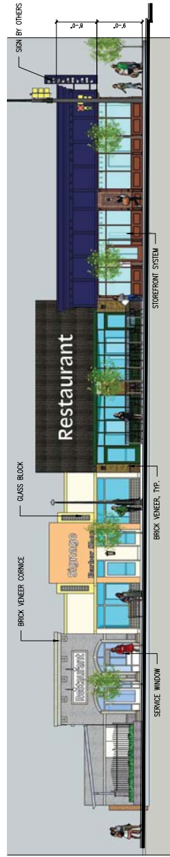
SOUTH EXTERIOR ELEVATION
