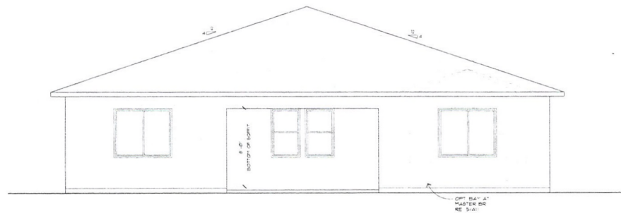
3 REAR ELEVATION E SCALE: 1/4"=1'-0" RE: A2.5A FOR ADDITIONAL NOTES & DIMENSIONS
