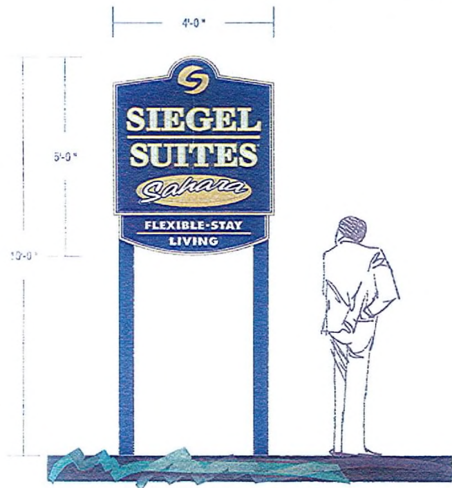
E DOUBLE FACED NON-ILLUMINATED WOOD SIGN WITH GRAPHICS SCALE 1/2"=1'
