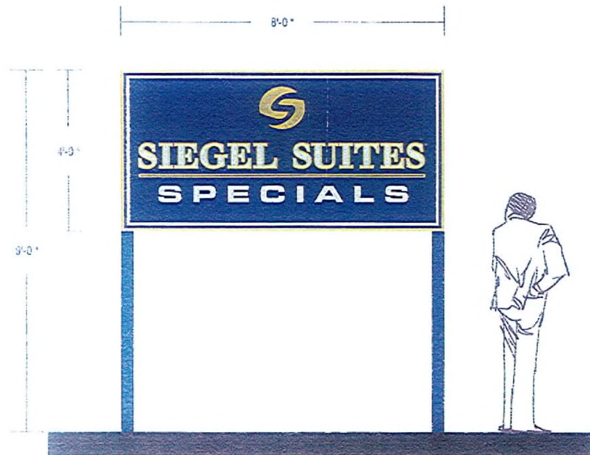
D DOUBLE FACED NON-ILLUMINATED WOOD SIGN WITH GRAPHICS SCALE 1/2" = 1'
