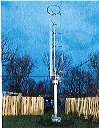
Ground-mounted vertical axis system Manufacturer: Windspire Location: North Carolina
