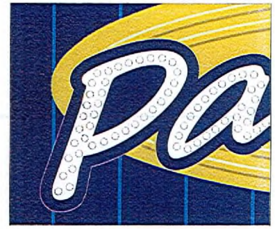
S-11 INCANDESCENT BULB DETAIL SCALE 3/4" = 1'-0" ANIMATION SEQUENCE...ALL BULBS SCINTILLATE
