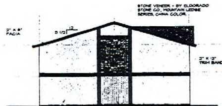
3 COAT 1/2" STUCCO OVER PAPER BACKED KEY MESH LATH (TYP. UN.) 2" x 2" VERT. TRIM 3 COAT 1/2" STUCCO IN VERTICAL SCORES @ 8" O.C. WEST ELEVATION (EAST ELEVATION IS OPP. HAND) SCALE: 1/8"=1'-0"
