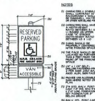
2 ACCESSIBLE PARKING SIGN SCALE: 1/2" = 1'-0"
