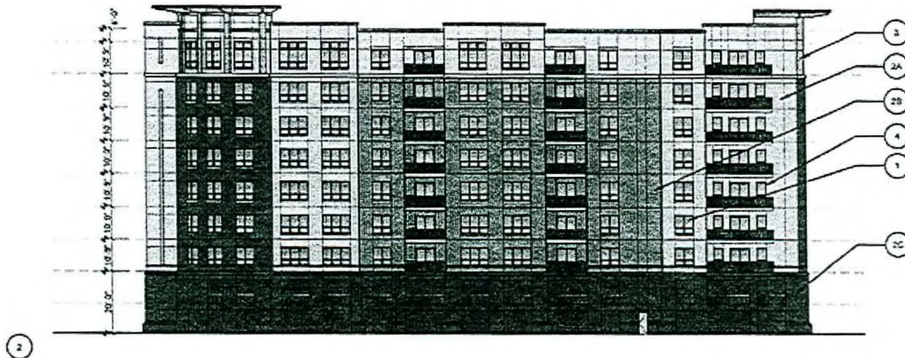
BUILDING 300 SIDE (NORTH & SOUTH) ELEVATIONS - BUILDING 200 SIMILAR 1/16"=1'-0"
