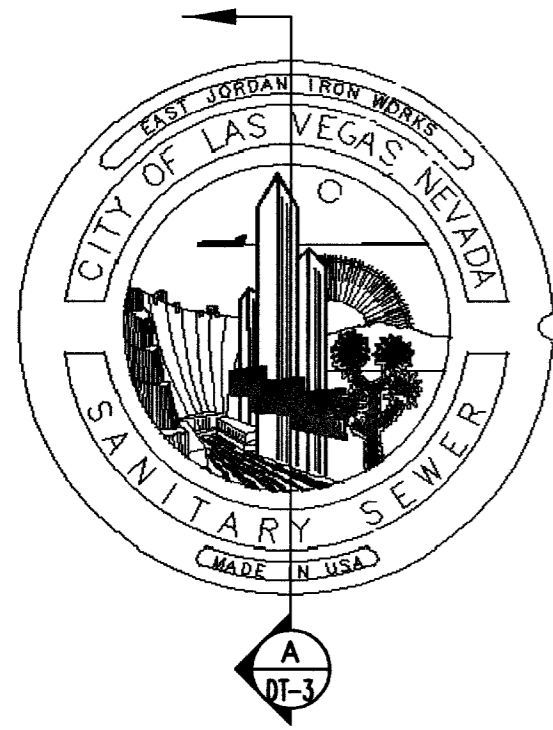
24" MANHOLE COVER PLAN VIEW
