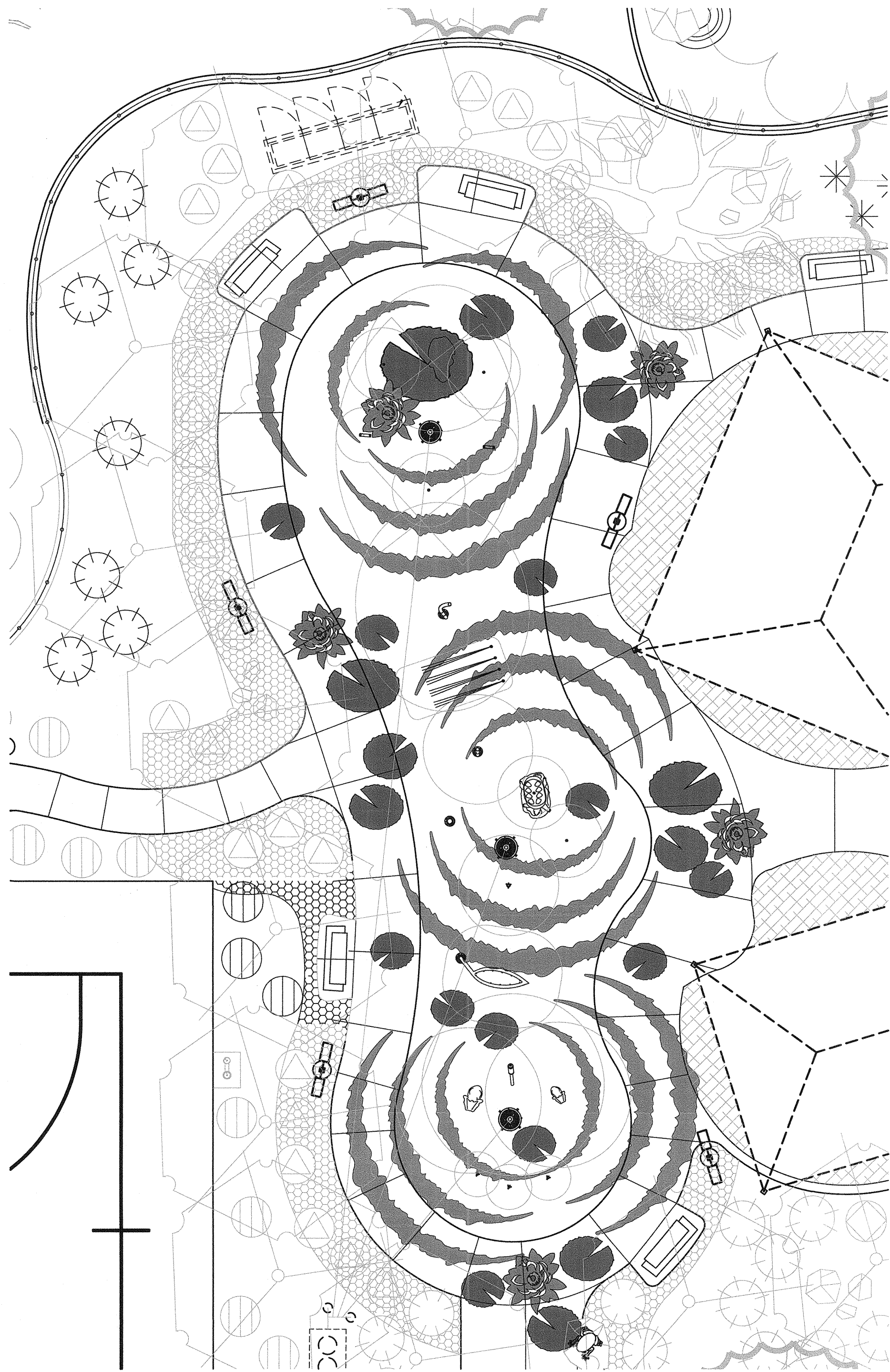
Enlarged Water Play Area - Colored Concrete Layout Scale: 1"=10'-0"
